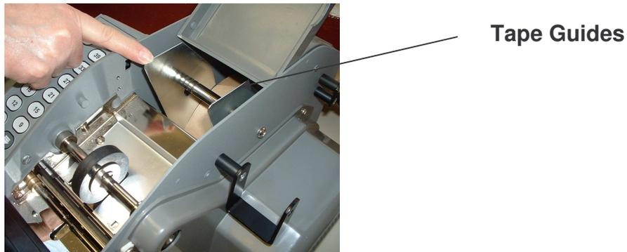
The tape roll guides should be properly set for the width of the tape being dispensed. The roll of tape should be center in the basket area and the roll guides adjusted loosely by lifting them and setting them on the desired pre-cut areas.
